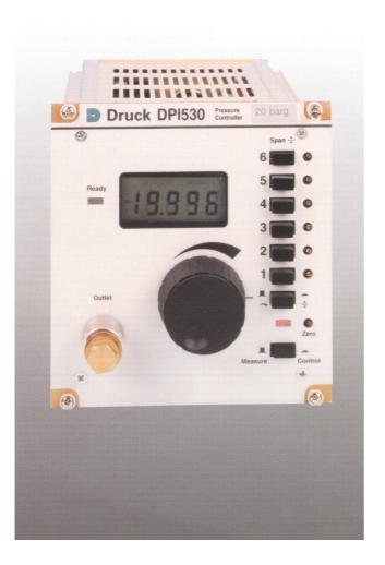
The DPI 530 is a fast response, digital closed loop pressure controller, using pulse width modulated valve technology. The controller is available with ranges up to 20 bar gauge or absolute and controls to an accuracy of ±0.1% F.S. with a stability of ±0.01% F.S.
