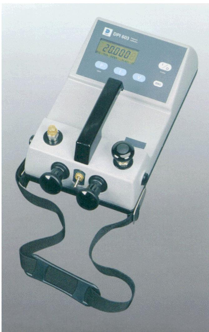
The cost effective DPI 603, which extends the Druck range of rugged portable battery powered pressure calibrators, has standard ranges of -1 to +1 bar, 2 bar, 10 bar or 20 bar gauge with an accuracy of  $\pm 0.075\%$
